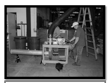
Above: Duct leakage testing in progress. Testing revealed not only significant leakage overall but also revealed an old HVAC IOM manual had been lodged against a VAV box primary airflow ring. The manual was blocking the majority of the duct free area and had been compromising control and zone comfort since original construction.
